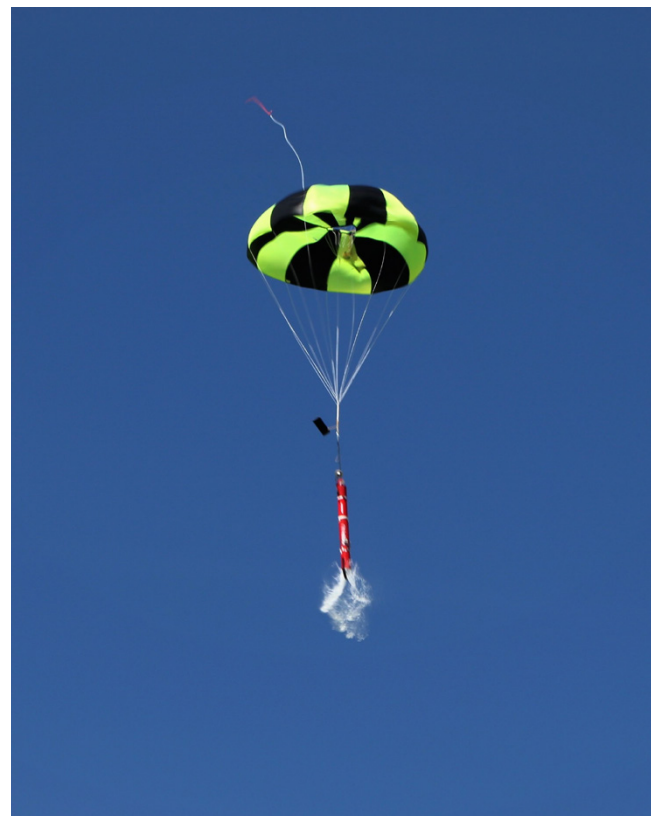
ANU-designed prototype water glider used to suppress fires while they are still small.
