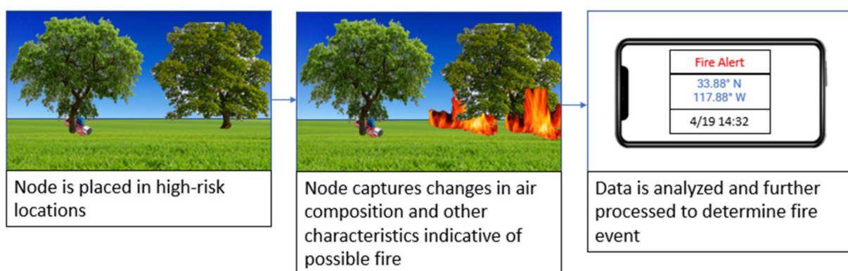
Figure 3. Basic sequence of operation for the majority of WSNs. Many may not share the exact steps but will follow these core functions. (Images sourced from Creative Commons, following the guidelines on Attribution 3.0 Unported, CC By 3.0 [26]. The only modifications to the images are cropping and resizing).
